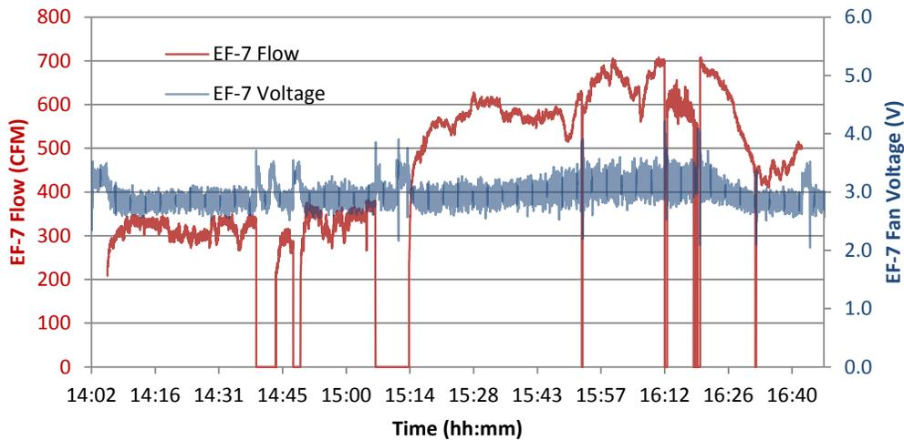
**Figure 79. EF-7 measured flow (cfm) and control voltage (1-s data)**
