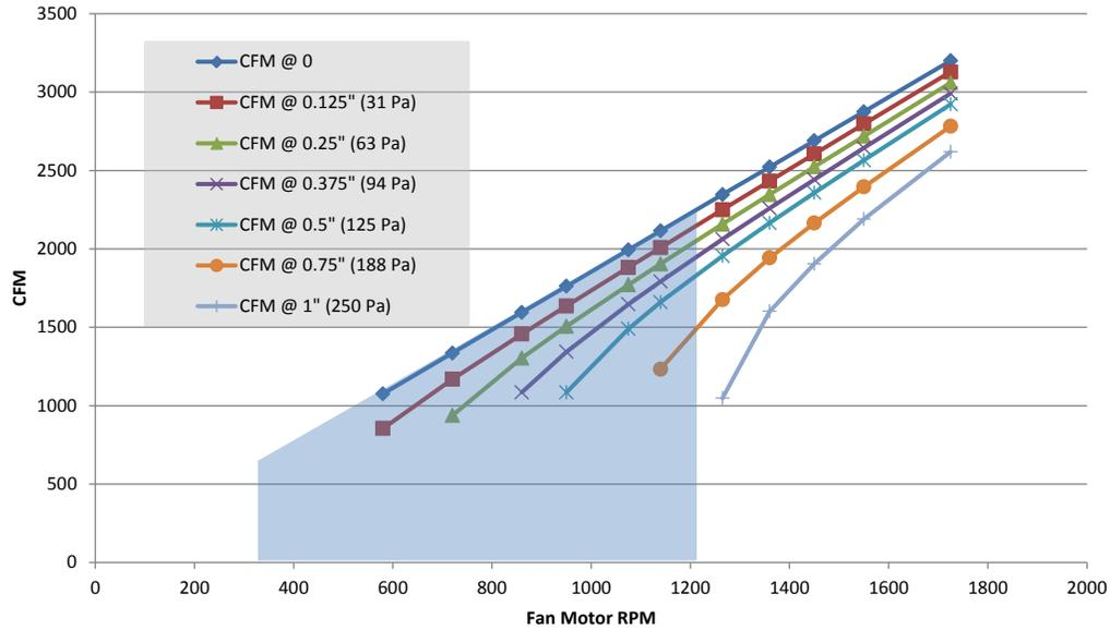
**Figure 78. Greenheck motor rpm versus cfm at various static pressures (rpm range highlighted)**
