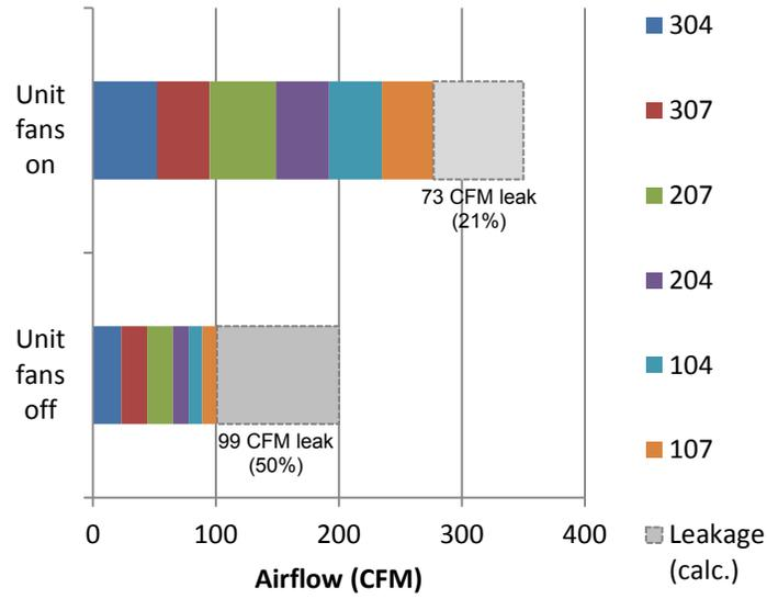
**Figure 67. EF-1 unit airflows and rooftop fan airflow (calculated duct leakage), turning unit fans on**
