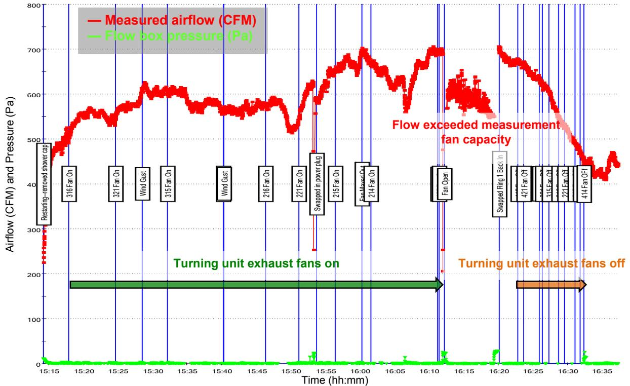
**Figure 58. EF-7 automated flow and pressure measurement (June trip test)**
