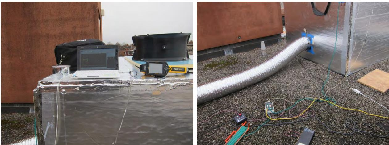
**Figure 54. Computerized flow capture hood testing (L), showing manometer (R)**
