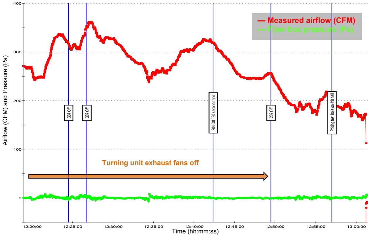
**Figure 59. Automated flow and pressure measurement (Day 2 test detail)**
