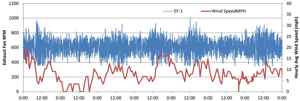
**Figure 84. EF-1 fan speeds for 02/03/12–02/09/12, showing diurnal variation**
