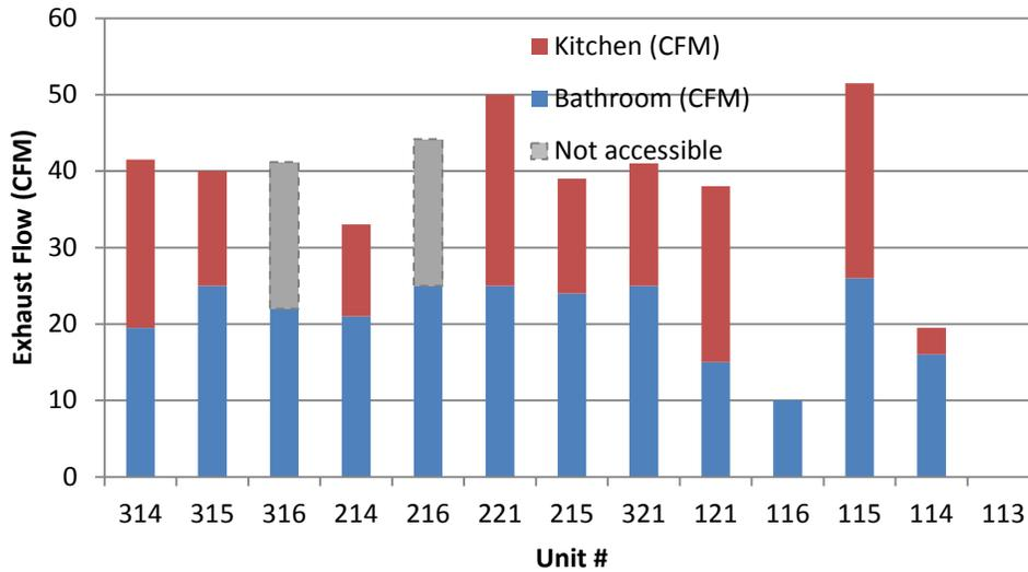
**Figure 66. Passive flow through unit exhaust fans (includes EF-6, EF-7, and EF-8 flows)**
