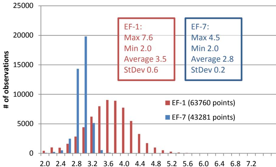
**Figure 85. Voltage measurement histogram for EF-1 and EF-7, with statistics**
