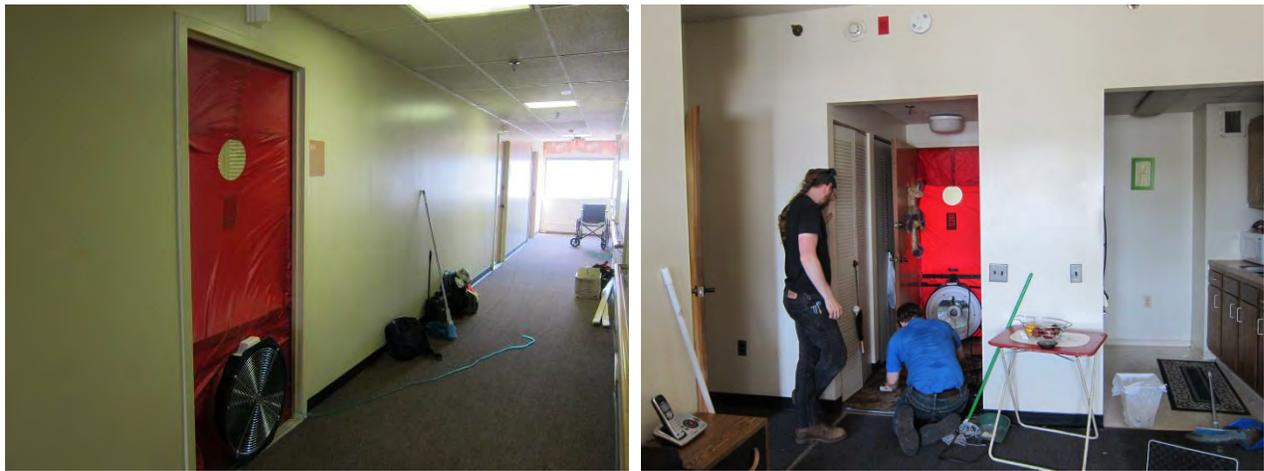
**Figure 43. Air leakage testing of units from hallway (L) and interior of unit (R)**
