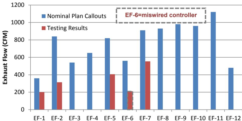
**Figure 60. Exhaust fan rooftop airflow test results**
