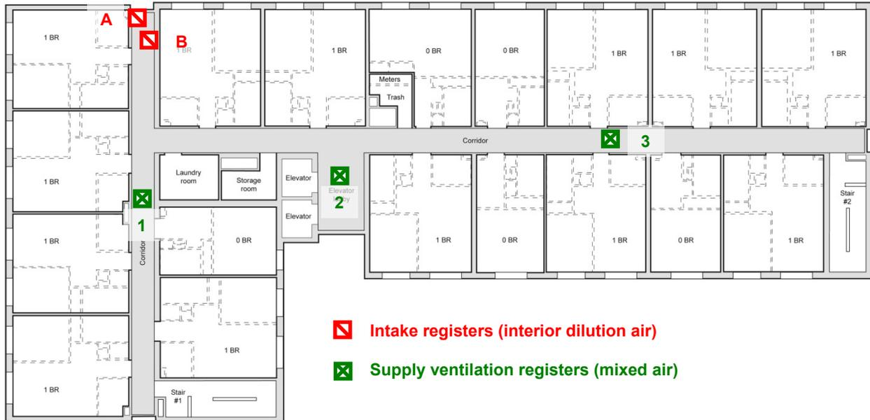
**Figure 90. Schematic of supply ventilation registers and interior dilution air intakes**
