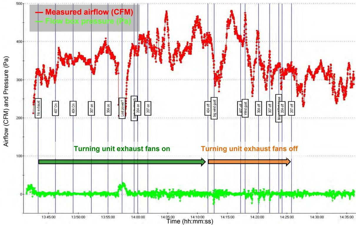
**Figure 57. EF-1 automated flow and pressure measurement (November trip, final test)**
