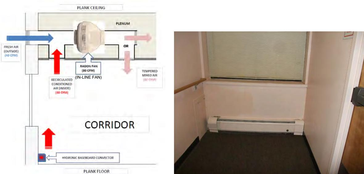
**Figure 23. Preliminary sketches of corridor ventilation (L), and corridor baseboard (R)**
