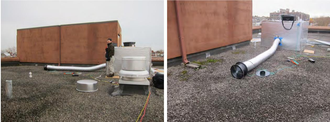
**Figure 53. Powered flow capture hood, showing duct testing fan**
