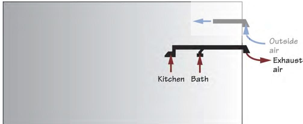
**Figure 18. Conceptual design of individual unit exhaust systems**
