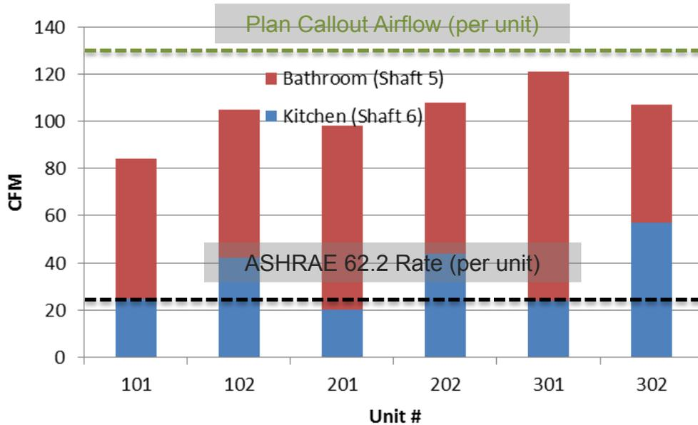
**Figure 40. Unit airflows for bathroom and kitchen exhaust fans, shafts 5 and 6**
