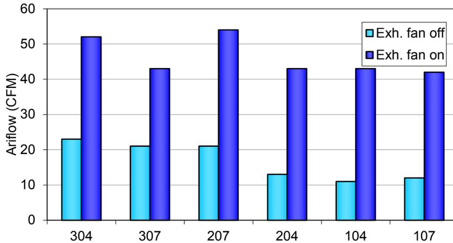
**Figure 63. EF-1 airflow measurement of individual unit exhaust fans, turning unit fans on**
