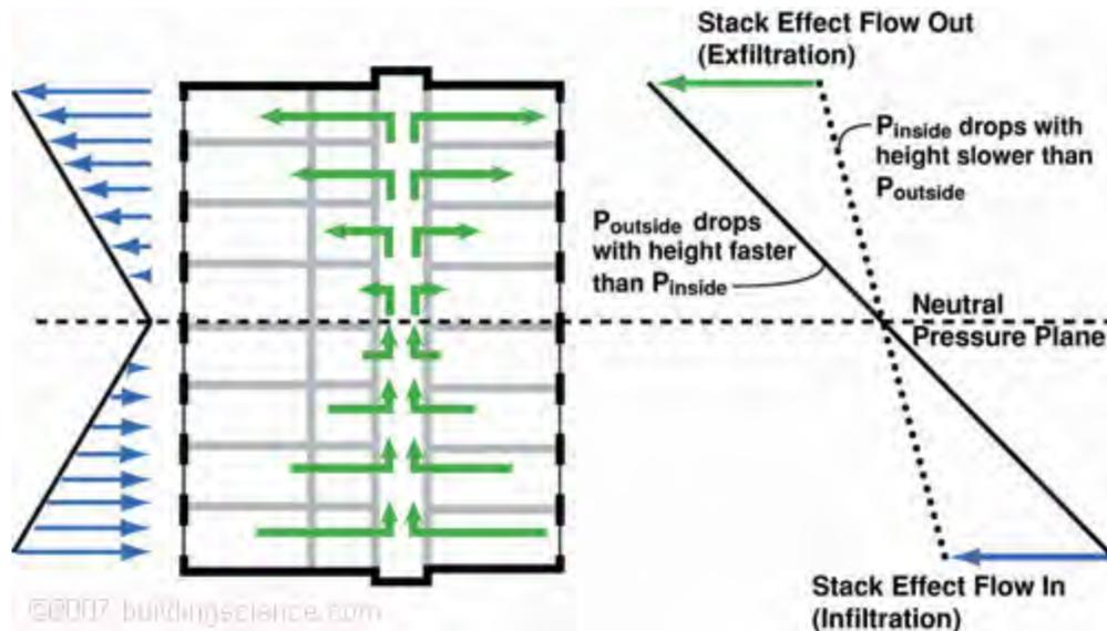
**Figure 3. Stack effect in multifamily buildings (simplified), showing shaft effects**
