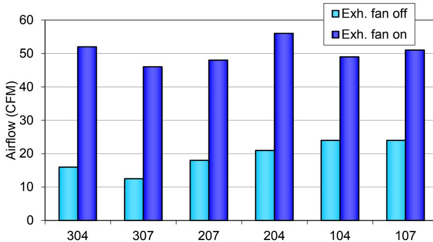
**Figure 64. EF-1 airflow measurement of individual unit exhaust fans, turning unit fans off**
