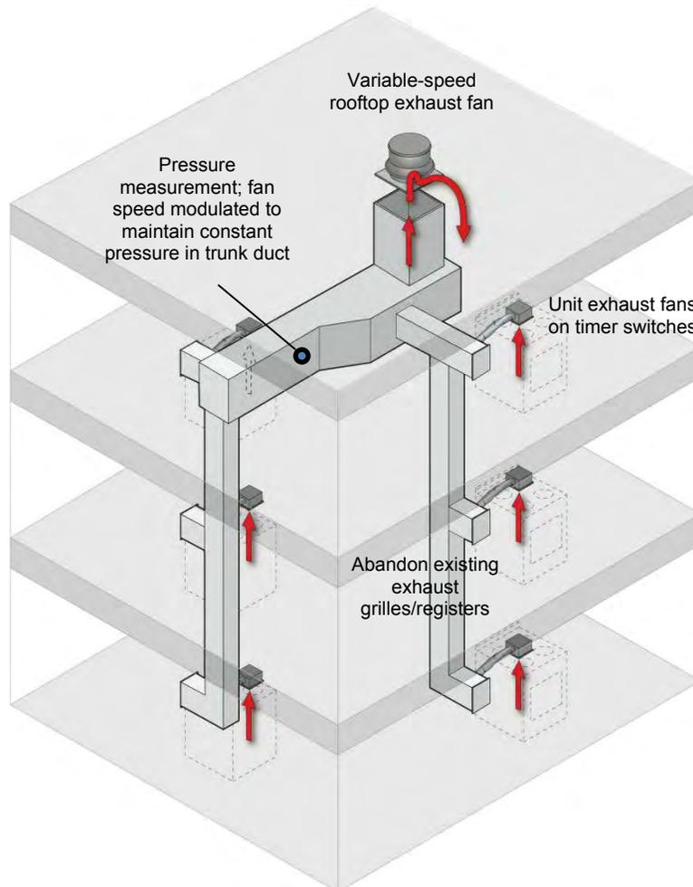
**Figure 21. Geometry of proposed exhaust system retrofit with individual exhaust fans**
