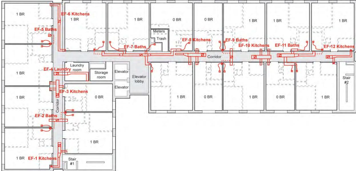
**Figure 16. Typical floor plan, showing kitchen/bath exhaust systems and risers**
