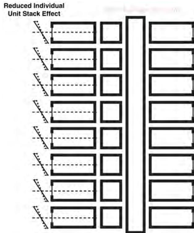
**Figure 4. Idealized compartmentalized multifamily building, showing stack per floor**
