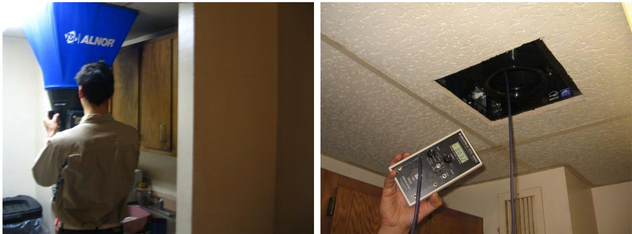
**Figure 62. Airflow measurement at kitchen exhaust fan (L) and duct pressure measurement (R)**
