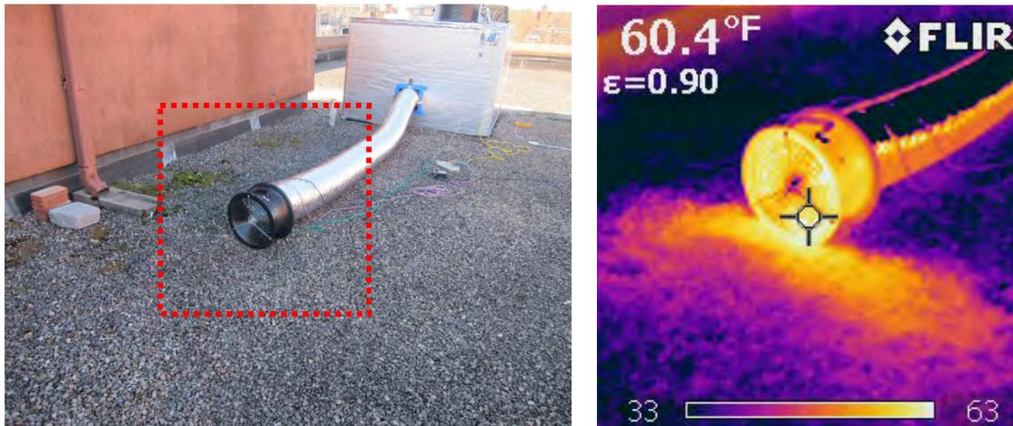
**Figure 56. Powered flow capture hood with infrared, showing output airflow heat signature**
