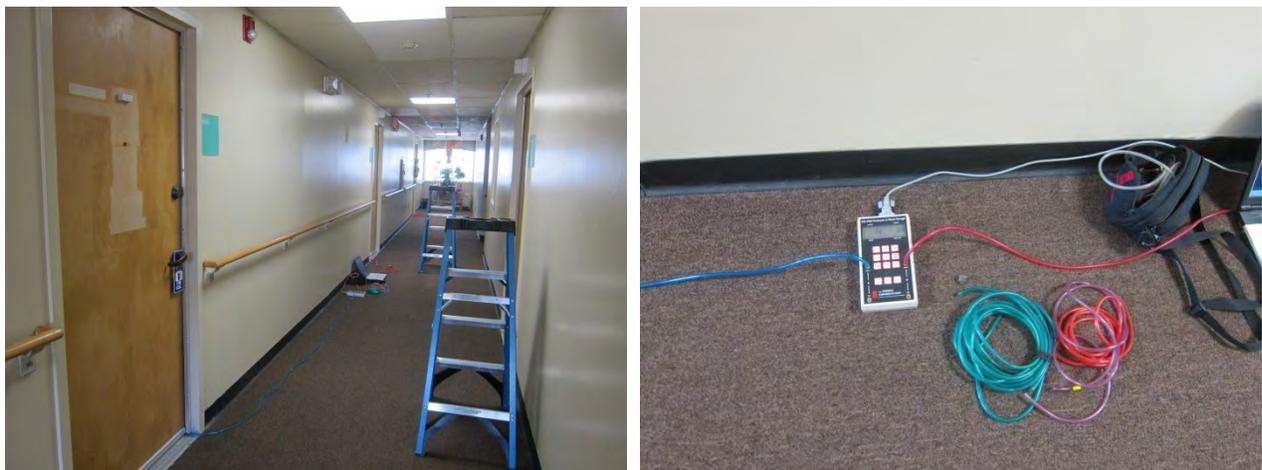
**Figure 74. Interunit pressure difference measurement**
