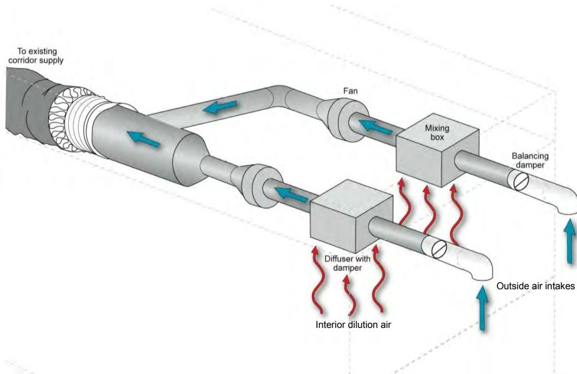
**Figure 86. Schematic of corridor ventilation system**
