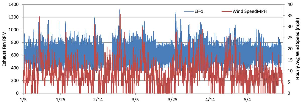
**Figure 81. EF-1 fan speeds with hourly exterior wind speeds for KPHL weather station**
