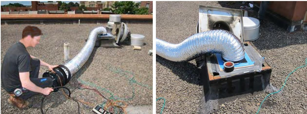
Figure 28. Air leakage testing of exhaust fan (EF) shaft 5 (EF-5)
