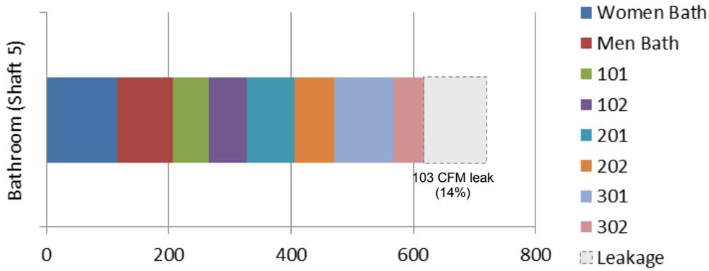
**Figure 42. Unit airflows compared to rooftop fan airflow, EF-5 (bathrooms)**
