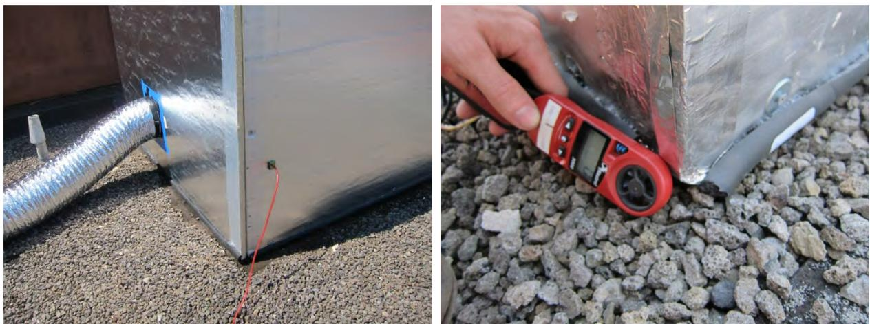
**Figure 35. Static pressure probe in enclosure (L); measurement of bypass leakage (R)**
