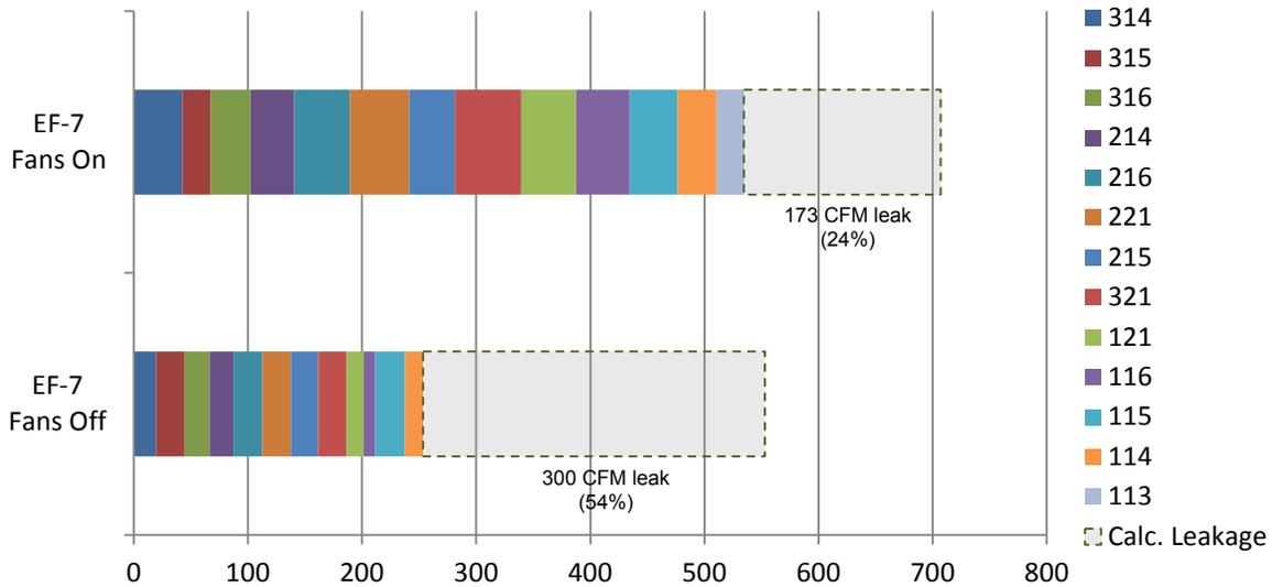
**Figure 69. EF-7 unit airflows and rooftop fan airflow (calculated duct leakage), turning unit fans on**
