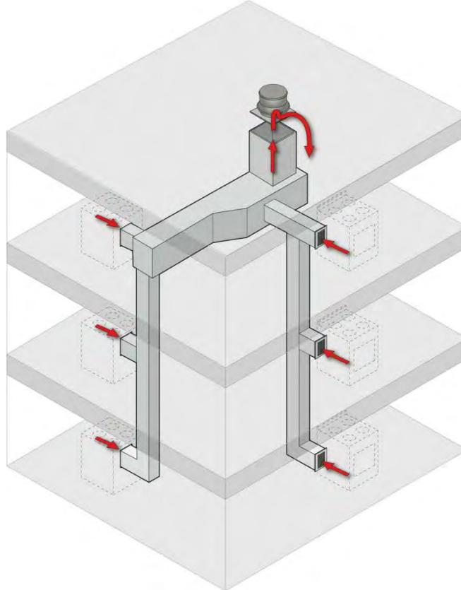
**Figure 38. Geometry of EF-1 (kitchen) shaft (six back-to-back kitchens)**
