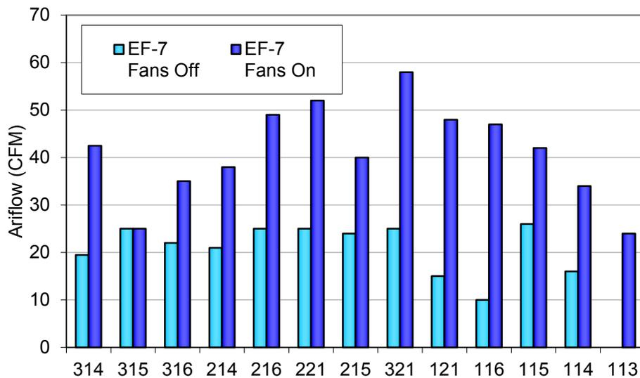
**Figure 65. EF-7 airflow measurement of individual unit exhaust fans, turning unit fans on**
