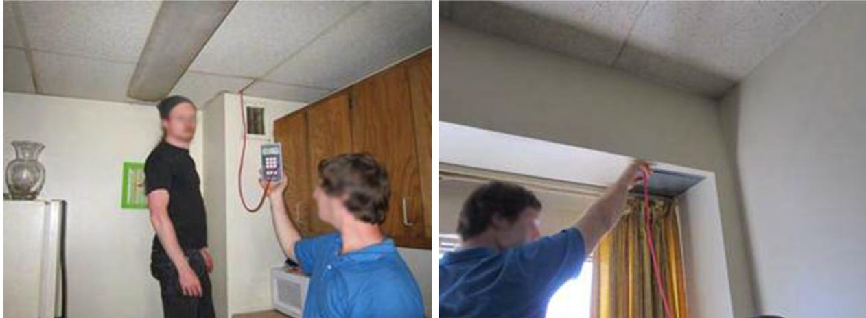
**Figure 45. Interzonal pressure measurements (suspended ceiling, L; mechanical access, R)**
