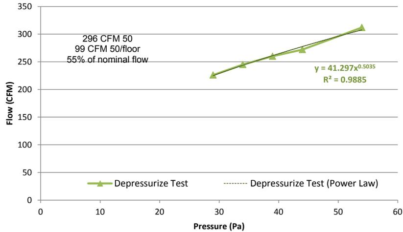
**Figure 73. Multipoint air leakage data for EF-3, post-retrofit**
