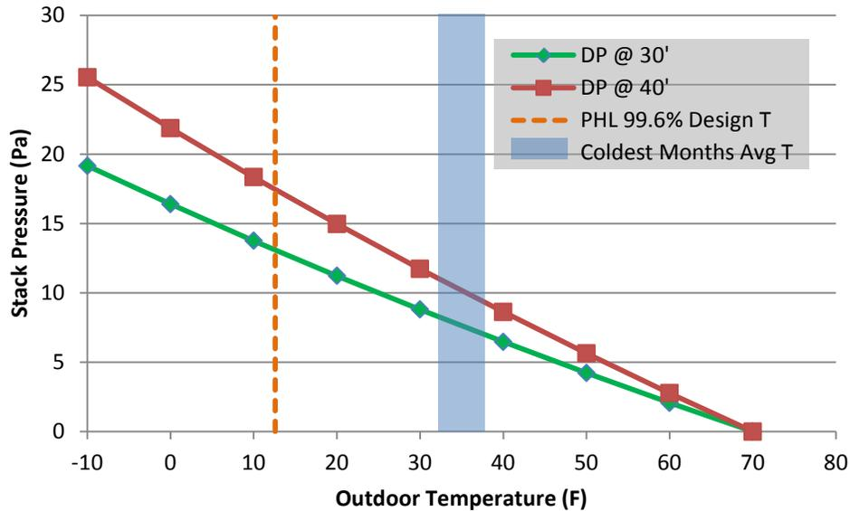
**Figure 6. Stack effect pressures for 30-ft and 40-ft heights, with Philadelphia weather conditions**
