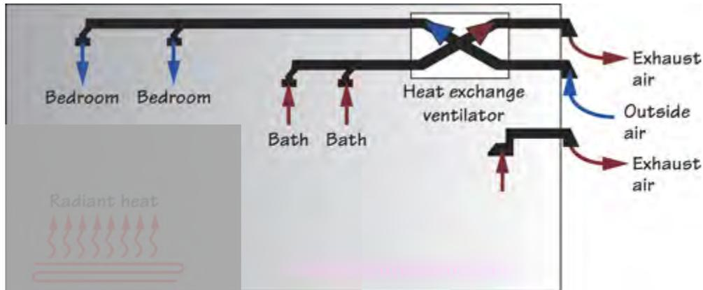
Figure 19. Conceptual design of individual unit HRV ventilation
