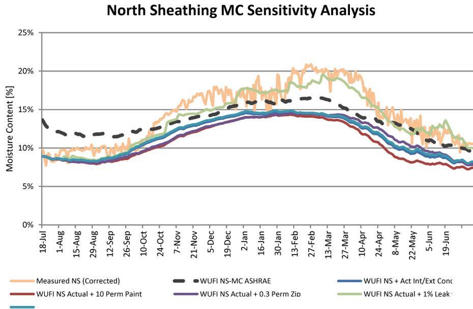
**Figure 3: Devens double stud north side sheathing MC vs. WUFI simulations (Arena 2014)**
