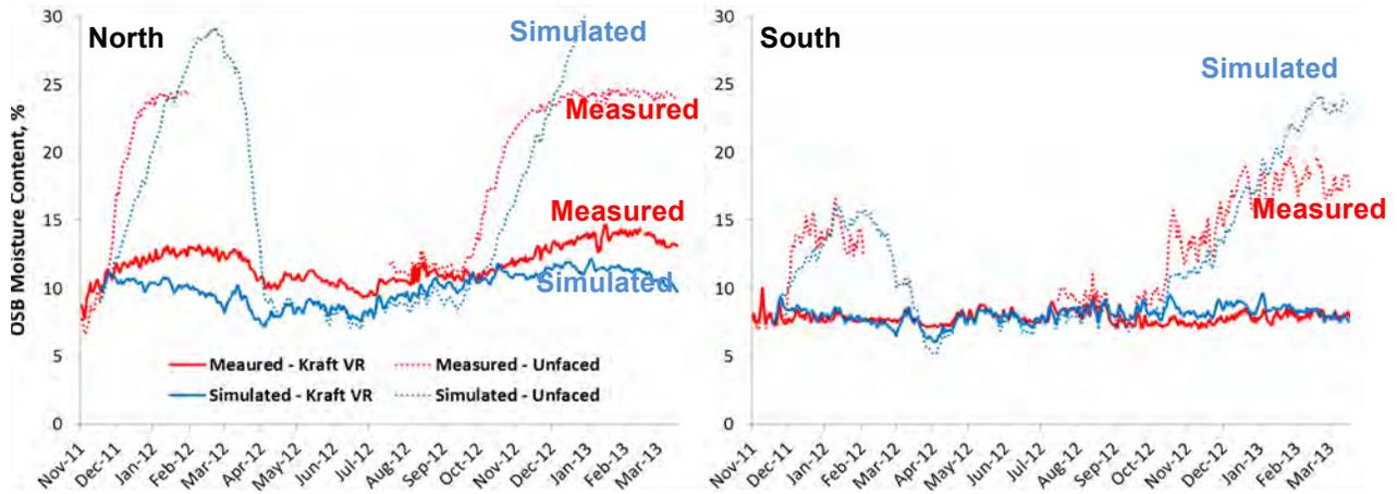
**Figure 6: Measured vs. modeled OSB MC, 2x6 w. vinyl siding (Glass 2014)**
