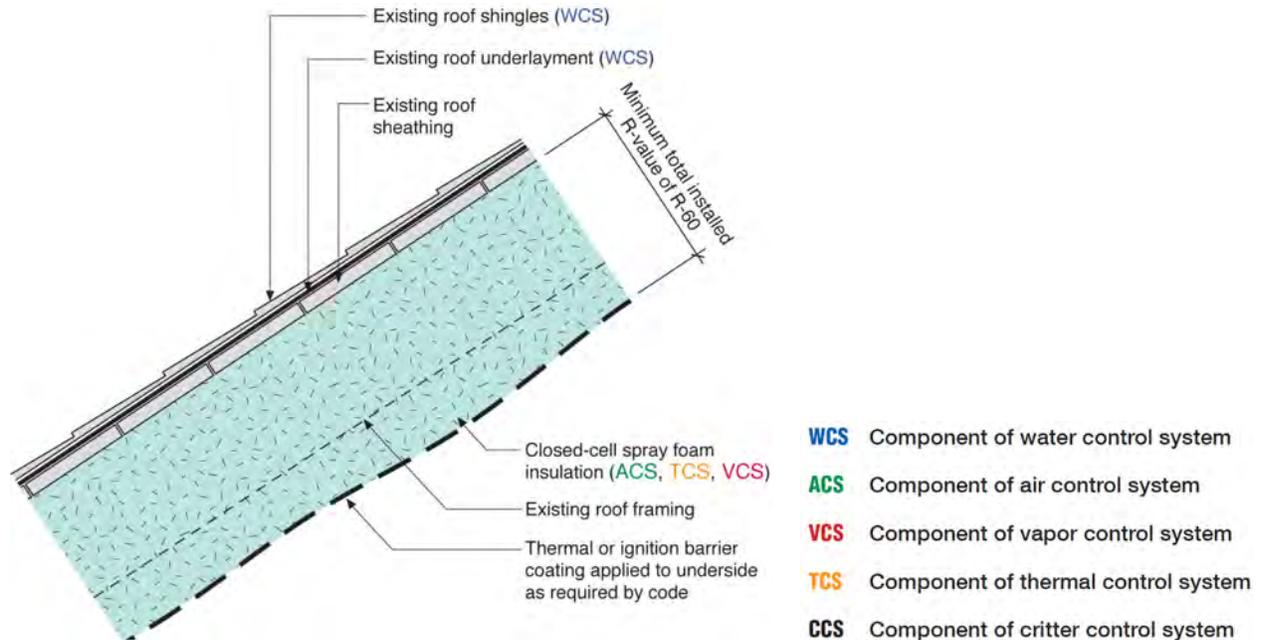
**Figure 9: Identification of control layers in an assembly (BSC 2013)**
