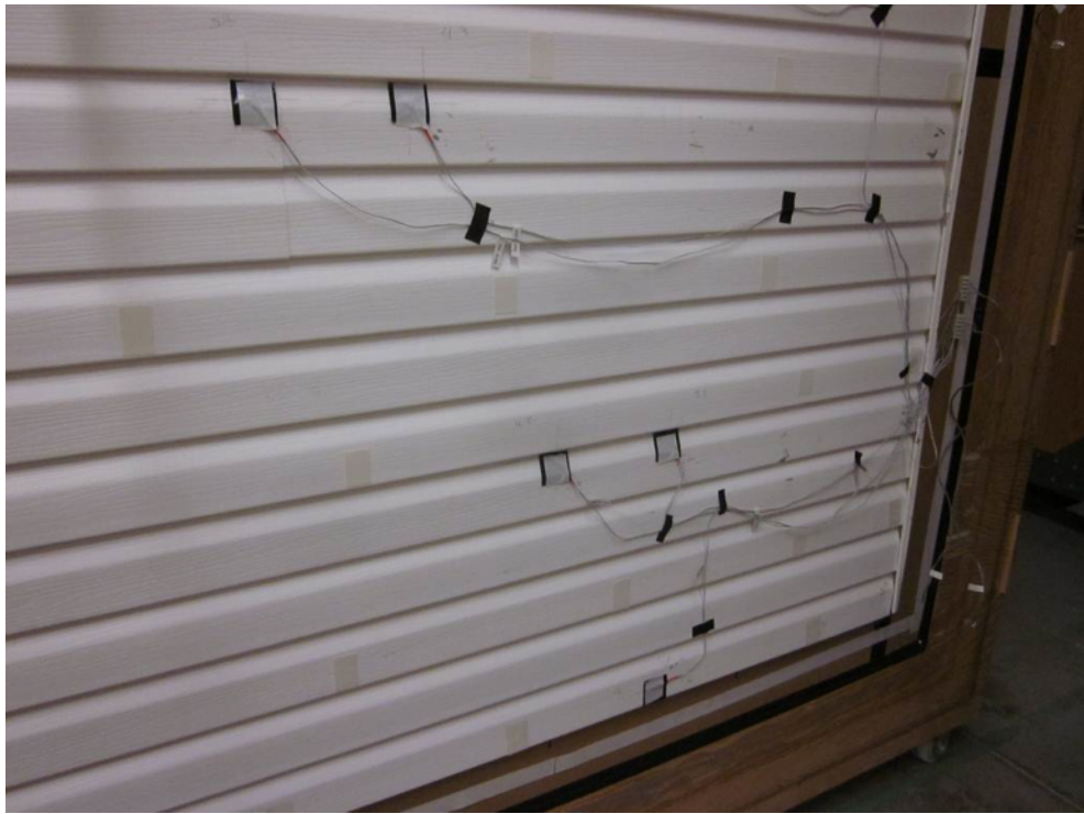
Figure 26 – Climate Box Side, Tape Grid
