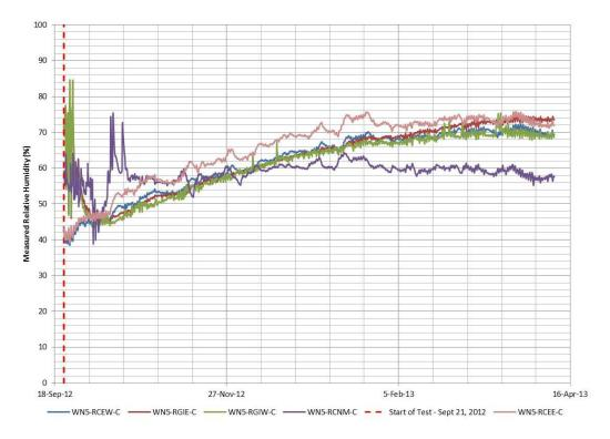
Figure 38 : North Wall 5 measured relative humidity
