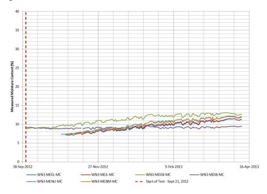
Figure 29 : North Wall 3 measured moisture contents
