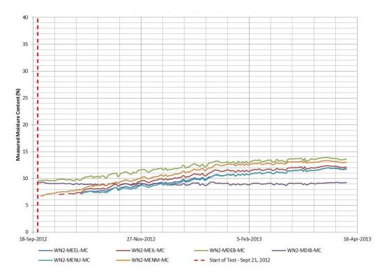
Figure 28 : North Wall 2 measured moisture contents
