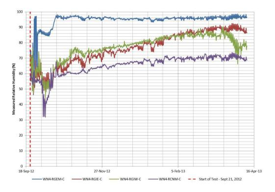
Figure 37 : North Wall 4 measured relative humidity
