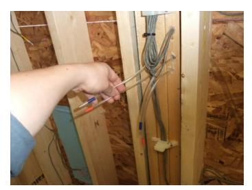
Figure 23 - Wetting Apparatus Injection Tubes
