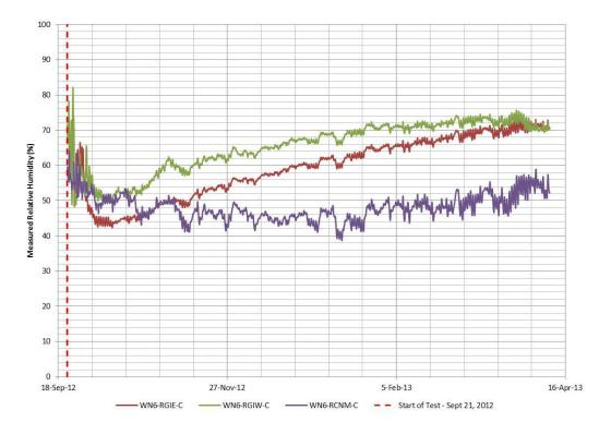
Figure 39 : North Wall 6 measured relative humidity
