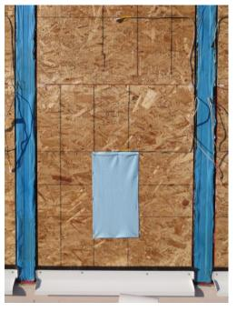
Figure 22 - Exterior Wetting Apparatus
