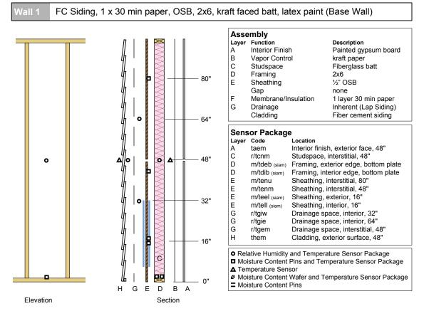
Figure 13 - Typical Instrumentation Package
