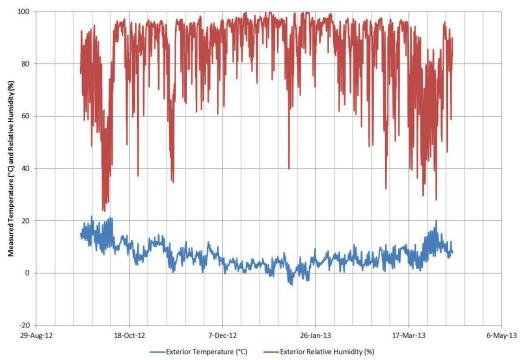
Figure 26 : Measured exterior temperature and relative humidity
