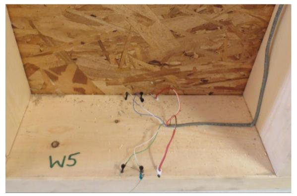
Figure 17 - Bottom Plate MC/T Sensors
