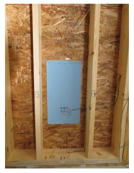
Figure 21 - Interior Wetting Apparatus
