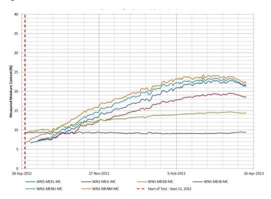
Figure 27 : North Wall 1 measured moisture contents
