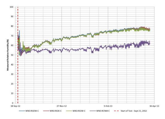
Figure 36 : North Wall 3 measured relative humidity
