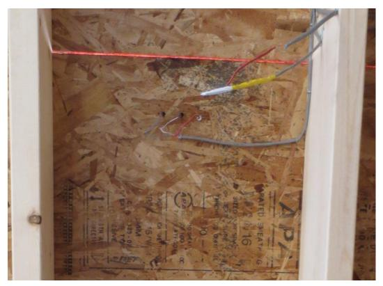
Figure 16 - Interior Mid-Height T, T/RH and MC/T sensors
