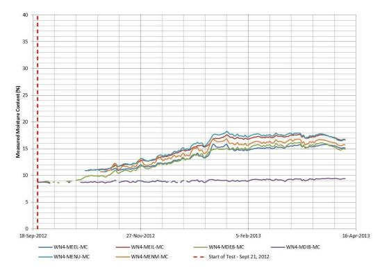
Figure 30 : North Wall 4 measured moisture contents
