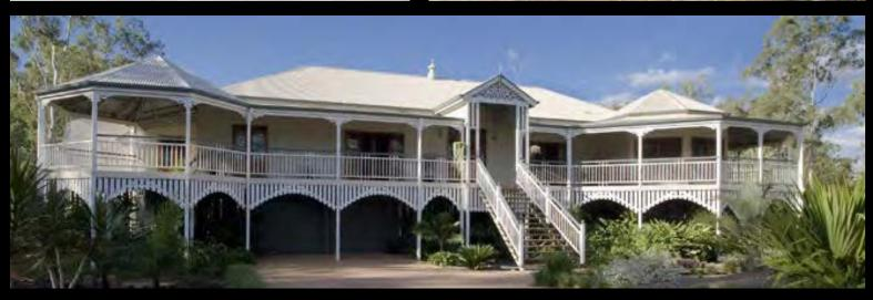
Decorated gal. ridge. ventilators Pyramidal roof Separate veranda Roll-down blinds Lattice front doors 0.07 Chamfer board cladding Note: simple hoods over side windows Lowset on stromps-Simple picket fence.
