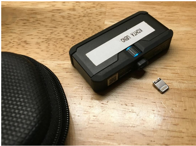
Figure 22: Breaking the connector off the FLIR ONE Pro
