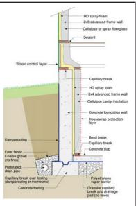
Figure 12: A hybrid approach for basement foundations can also be used in combination with fiberglass or cellulose insulation.
