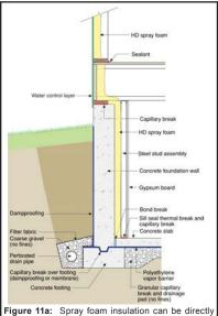
Figure 11a: Spray foam insulation can be direct applied to the interior of concrete foundation walls.
