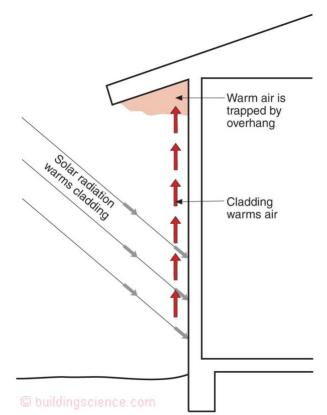
Figure 5: Cladding Thermal Plumes - Dark cladding, solar radiation and large over-hangs combine to create ice-dam heaven.
