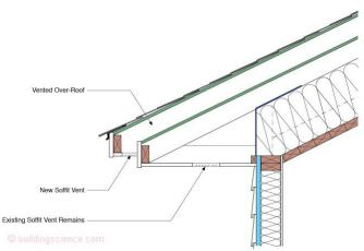
Figure 3: Vented Over Roof Soffit - The best approach is to over roof. Add a vented roof over the top of the existing roof. The vented over roof needs to be extremely well vented. We are not able to deal with improving airtightness to any real degree and we can't add much thermal insulation to any real degree so removing the heat using ventilation is the only thing left in the tool box.
