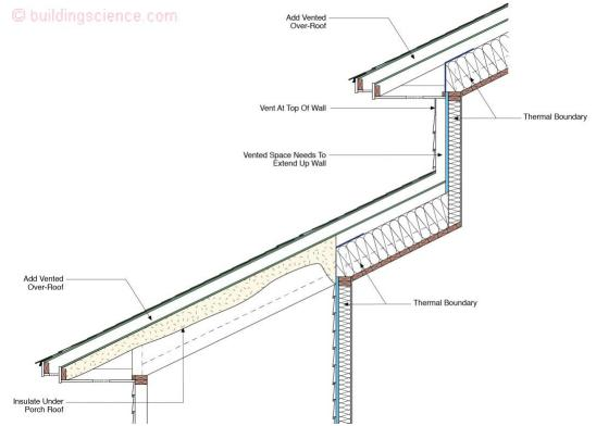
Figure 6: Venting Up The Wall - Insulate the projecting overhang with spray polyurethane foam (SPF) and over roof. Where the over roof vent intersects the wall run the vent up the wall...you need to "over wall" create a vented wall...like a "rain screen"...but bigger... a "vent screen" October 2018
