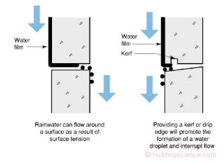
Figure 2: Surface Tension – A driving force for rain entry.
