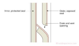
Figure 12: Two-Stage Joint Section - Section through a two-stage joint that uses sealant to direct water to the exterior.
