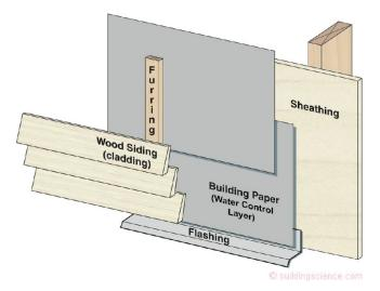
**Figure 9:** Drained Assemblies - Drained assemblies have multiple layers dedicated to water management. An example of a drained assembly is a wood frame wall with oriented strand board sheathing (OSB) covered with building paper and clad with wood siding on furring.
