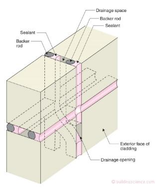
**Figure 13**: Three Dimensional Detail of Two-Stage Joint - Drainage paths are shown. The outer seal is exposed to the elements – ultra violet light, heat and water – but the assembly still works because of the interior protected seal.
