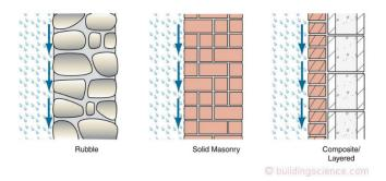
Figure 8: Mass/Storage - Rainwater entry controlled by providing materials that can store, absorb, redistribute and dry (Courtesy of Straube, 2012).
