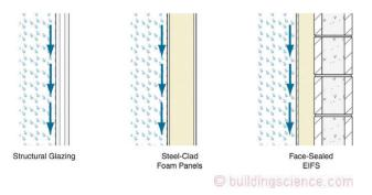
Figure 7: Barrier - Rainwater entry prevented by providing a barrier (Courtesy of Straube, 2012).
