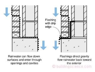
Figure 1: Gravity – A driving force for rain entry.
