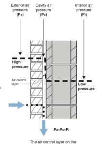
The air control layer on the masonry wall reduces the air pressure driving force across the brick
