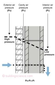
Driven by air pressure differences, rain droplets are drawn through wall openings from the exterior to the interior
