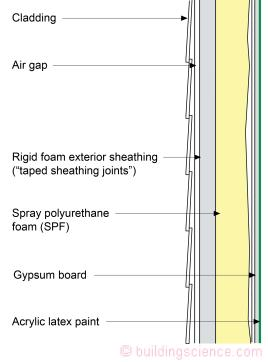
Notes: High density closed cell foam can be used in all IECC Climate Zones. Where low density open cell foam can be used the thickness or thermal resistance of the rigid foam exterior sheathing is specified by the International Residential Code (IRC) based on Climate Zone and the thickness of the wall framing.
