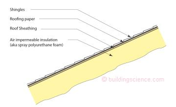
**Figure 5:** Unvented conditioned attics can be constructed by installing low density open cell or high density closed cell spray foam directly to the underside of the roof deck.
