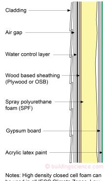
Notes: High density closed cell foam can be used in all IECC Climate Zones. Low density open cell foam can be used in IECC Climate Zones 1 through 4 without an interior vapor retarder.
