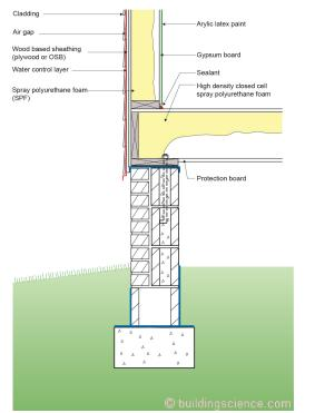
Figure 14: A protection board such as fiber cement should be installed to prevent animals from getting into the floor assembly.
