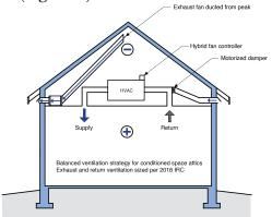
**Figure 10:** The best way to remove moisture from the attic space is to provide air change. Air is exhausted from the peak of the attic using an exhaust fan ducted to the exterior.
