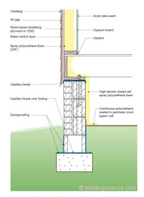
Figure 15: Conditioned crawlspaces should be constructed as "mini" basements and completely connected to the house.
