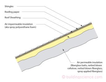
Figure 7: A further variation of hybrid attics is where the low-density open cell spray foam is replaced with fiberglass or cellulose insulation.
