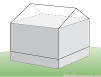
**Figure 1:** Houses have walls, roofs and foundations that each have to be connected to each other providing continuity of the water control layer, air control layer, vapor control layer and thermal control layer.
