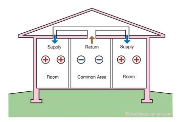
Figure 1: HVAC System Pressures – Typical pressure difference between bedrooms and common areas in houses with forced air distribution systems.
