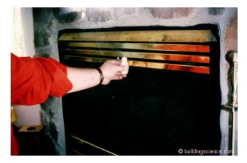
**Photograph 5: Backdrafting Gas Fireplace** - Soot from standing pilot lights on gas fireplaces are a big source of particulates. When the full burners are on venting occurs. When only the pilot light is on backdrafting is common.
