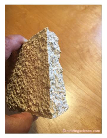
Photograph 9 – Coating on Back of Manufactured Stone Veneer: Manufactured stone is back-coated ("sealed") to prevent excessive water absorption out of the thin set. The issue is desiccation of the polymer modified thin set mortar leading to not establishing a bond. So a "porous" not real stone is made to behave like a non-porous real stone with the back-coating.
