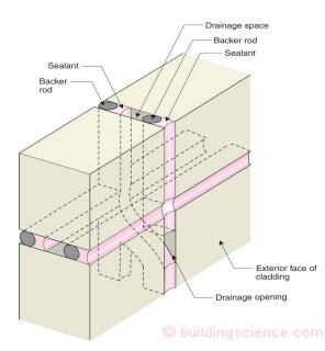
Figure 1: Two-Stage Joint - Precast panel assemblies as well as concrete tilt-up systems employ two-stage joints that facilitate drainage. We have the precast industry for this innovation from the 1950's and from a legend by the name of Kirby Garden of the Division of Building Research of the National Research Council of Canada
