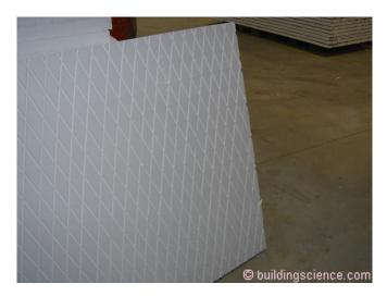
**Photograph 6: Drainage Grooves** – Channels cut into the back of expanded polystyrene (EPS) to provide drainage. This comes to us from New Zealand. Apparently the Kiwis have heard of Vitruvius.
