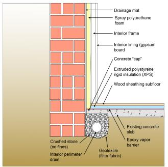
**Figure 6:** Avoiding Interior Vapor Barriers – Part I – Interior insulation layer can dry inwards from the face of the airtight and vapor tight interior drainage layer. In this assembly a drainage matt is insulated with spray polyurethane foam.
