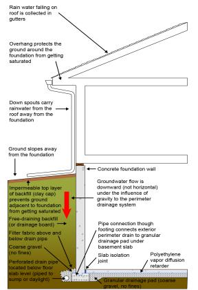
**Figure 3: Drain the Ground** - You have to keep the ground water from getting to your basement foundation walls. Start with providing an impermeable layer covering the ground adjacent to basement foundation. Then provide a free draining layer of backfill material so that the penetrating groundwater is directed downward to a perimeter drain.
