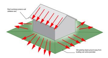
**Figure 2: Drain the Site** - Drain the water away from foundation perimeters. Keep "surface water" from becoming "ground water". Roof and façade water should not saturate the ground beside foundations. Grade should slope away from building perimeters.
