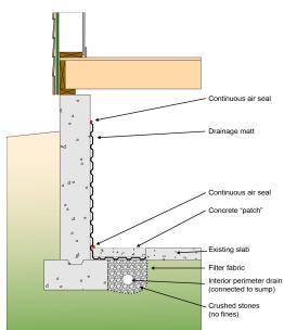
**Figure 5: Interior Drainage System** - You don't have to dig up the exterior and re-landscape when you install an interior perimeter drain and couple it with a full height interior drainage layer. This drainage layer needs to be vapor tight and airtight to control the entry of water vapor and soil gases.
