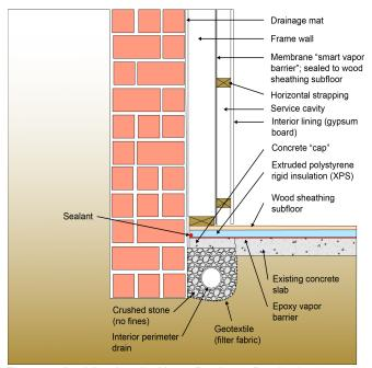
**Figure 7:** Avoiding Interior Vapor Barriers – Part II – Interior insulation layer can dry inwards from the face of the airtight and vapor tight interior drainage layer through the membrane "smart vapor barrier". Note that the "smart vapor barrier" becomes vapor open as the relative humidity the membrane "sees" goes up. The typical inflection point for most "smart vapor barriers" is between 40 percent and 70 percent relative humidity.
