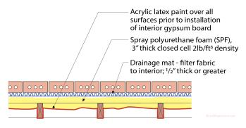
Figure 6: More Spray Polyurethane Foam - The SPF
