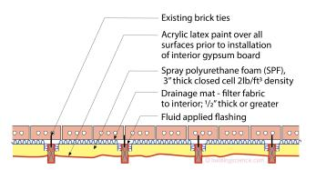
Figure 7: Brick Ties Get To Stay - Note the wrapping of the outside of the studs with the fluid applied flashing. The SPF needs to adhere directly to uncoated wood...you need to stop the fluid applied flashing "exterior wrap" to leave enough exposed wood stud for full SPF adhesion.
