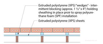
**Figure 3: Wedges** - The XPS is "wedged" in place with XPS wedges at stud locations. The thin flexible XPS sheet is "fished" in behind the studs with the wedges holding it in place. That is why the brick ties needed to disappear. The XPS sheet needs to be limited in height to probably no more than three feet to allow the wedges to be "smushed" into place from the top downwards.
