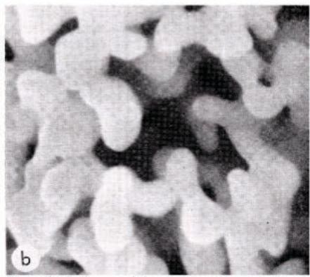
Figure 1b. Brick, sintered clay, porosity 40 per cent.
