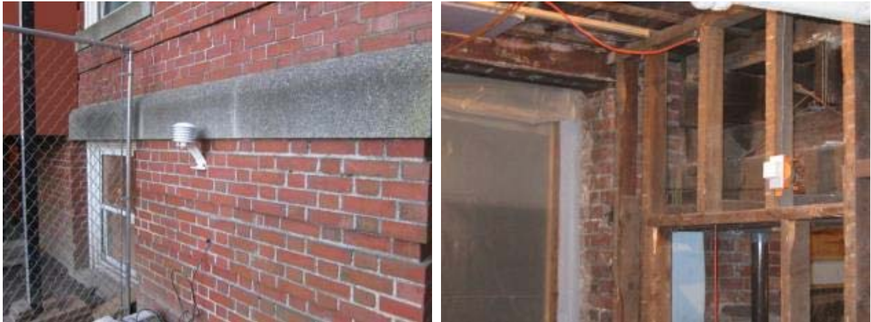
Figure 36. Exterior (left) and interior hallway (right) temperature and RH sensors
