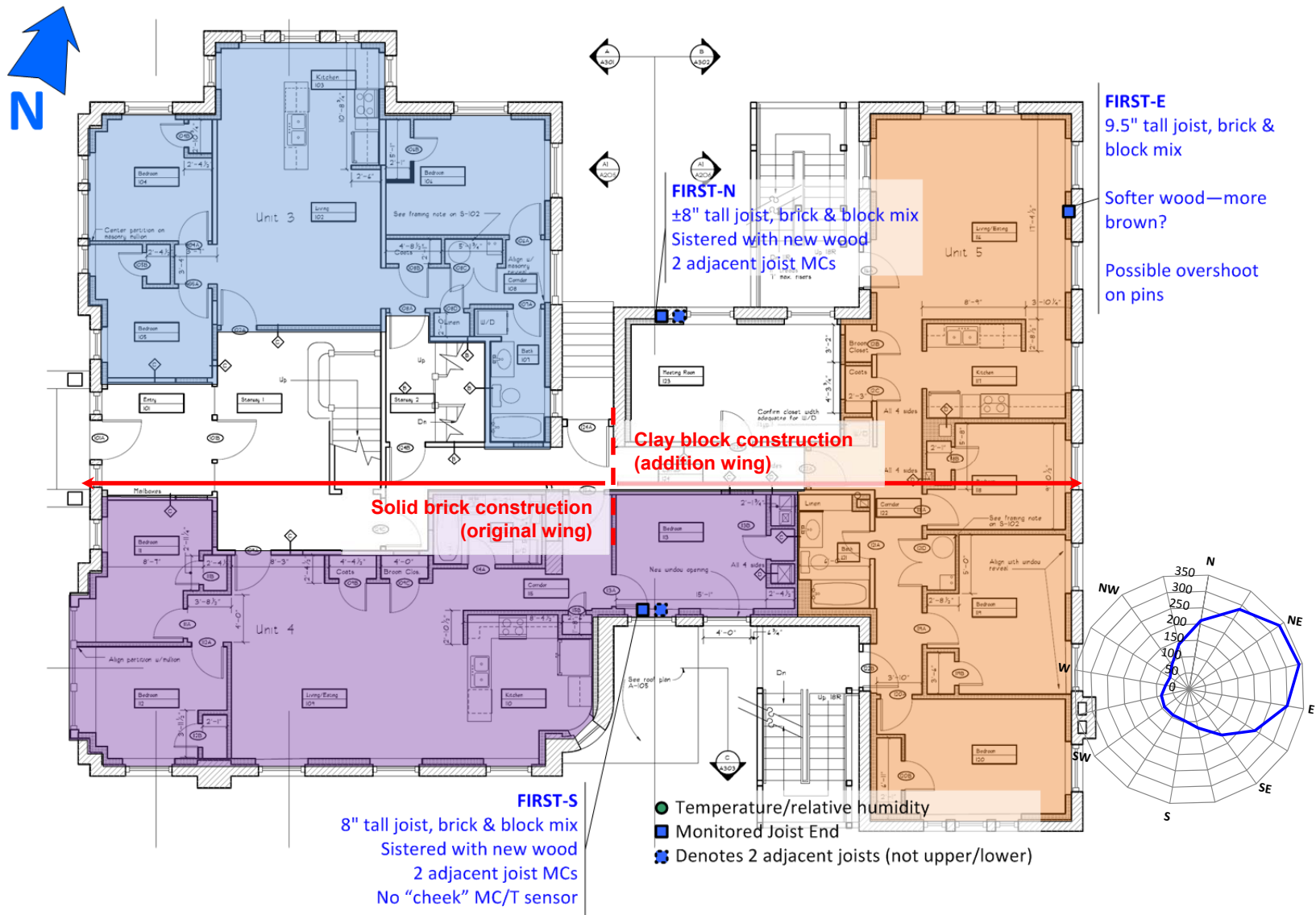
Figure 22. Location of monitored joist ends at first floor (first-floor ceiling) with driving rain; residential units highlighted
