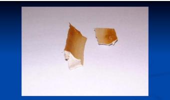
**Problem:** Sealant discoloration **Solution:** Isolate from contact with asphaltic waterproofing membrane
