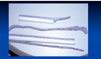
**Problem:** Bubbles in sealant **Solution:** Do not puncture closed cell backer rod or use a different backer rod type
