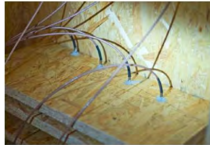
Figure 6: "Modules" that could each hold two ducts to which the illmod Trio was applied. The left picture shows the front aspect that faced the refrigerator with expanded illmod 600 used as a sealant. The right picture shows the posterior aspect that faced the climatic chamber. The illmod Trio was applied and the four sensors installed for recording. Left picture taken on 2 nd Jun 2010, right picture taken on 14 th Jul 2010.
