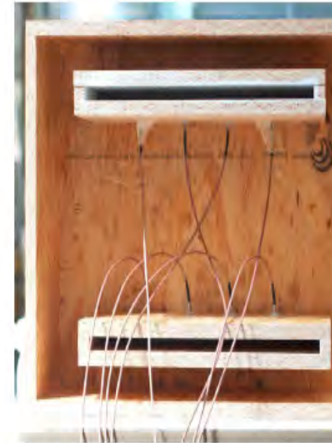
Figure 6: "Modules" that could each hold two ducts to which the illmod Trio was applied. The left picture shows the front aspect that faced the refrigerator with expanded illmod 600 used as a sealant. The right picture shows the posterior aspect that faced the climatic chamber. The illmod Trio was applied and the four sensors installed for recording. Left picture taken on 2 nd Jun 2010, right picture taken on 14 th Jul 2010.
