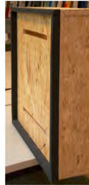
Figure 6: "Modules" that could each hold two ducts to which the illmod Trio was applied. The left picture shows the front aspect that faced the refrigerator with expanded illmod 600 used as a sealant. The right picture shows the posterior aspect that faced the climatic chamber. The illmod Trio was applied and the four sensors installed for recording. Left picture taken on 2 nd Jun 2010, right picture taken on 14 th Jul 2010.
