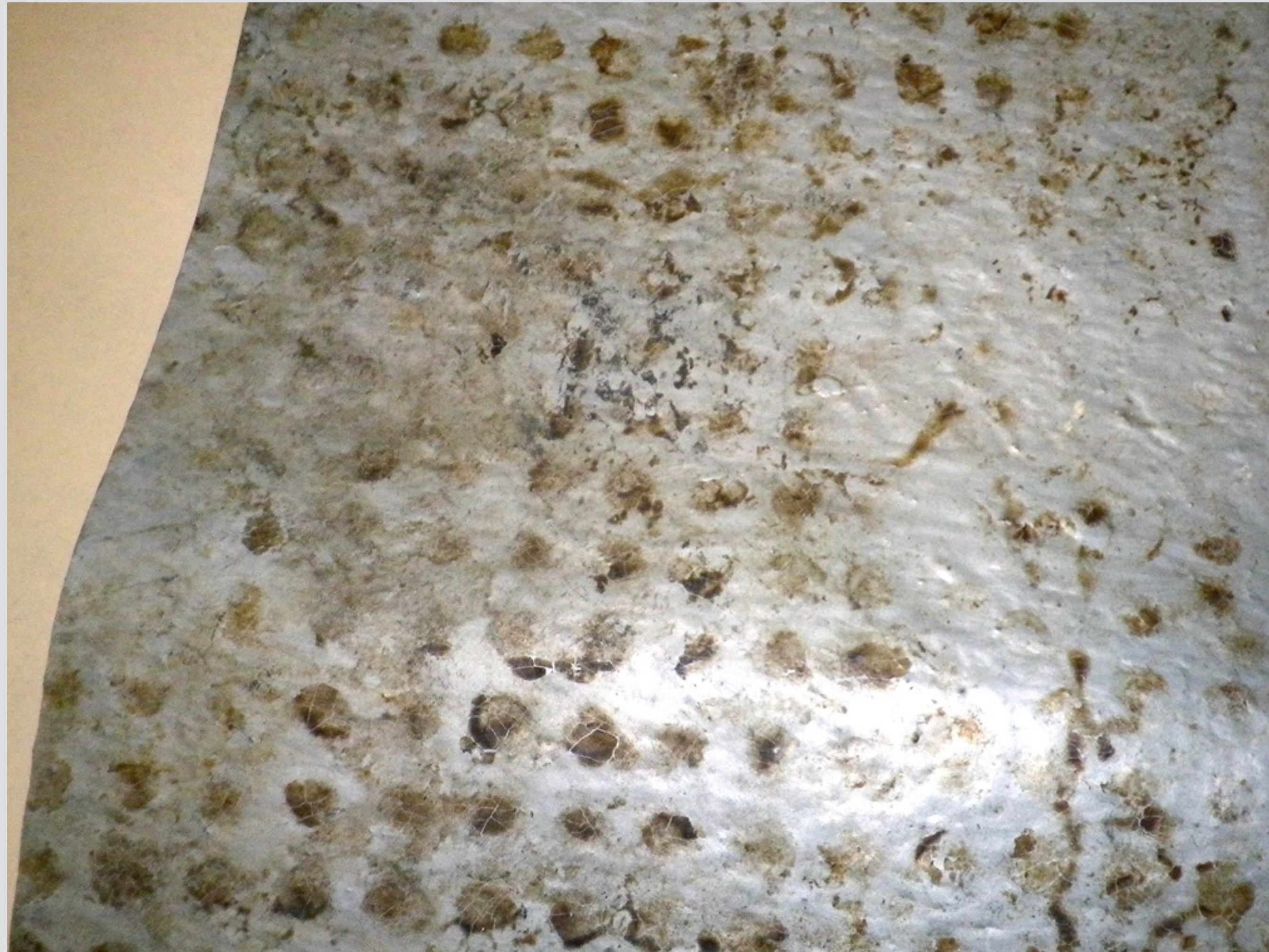
Fully reinforced liquid applied roof 1998. Removed this section in August 2014 to see how it was holding up. It looks good after 17 years, but can we get another 20/25 years out of it?
