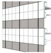
Step 1: Existing marble panels are removed
