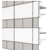
Step 8: USP curtainwall and trim is installed
