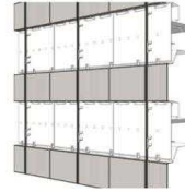
Step 4: Window washing tracks are removed
