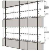
Step 3: Existing marble support clips are removed
