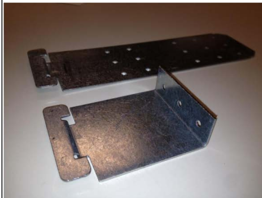
Photo #2 Standard Installation Clip is cut to length and then bent 90°. The clip length will need to be determined per job as it is based on the width of the joint between the sill dam and the window plus the leg height of the sill dam.
